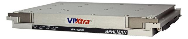
Inputs:28VDC or 48VDC or 270VDC or AC single or 3 phaseOutputs:12VDC @ up to 80A5VDC @ up to 80A3.3VDC AUX @ up to 40A+/-12VDC AUX @ up to 1.5A+/-12VDC AUX @ up to 1.5APower Max:1528WDissipation: up to 200W
